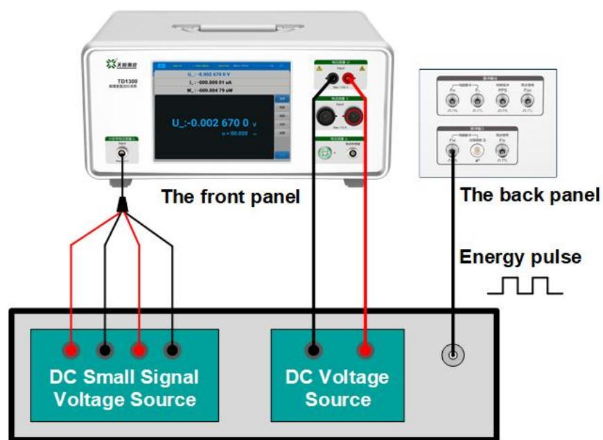
**Verification Equipment for Indirect Connected DC Electrical Energy Meters (DUT)**
