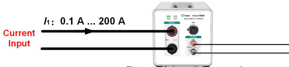
Figure (a) Schematic diagram of direct connection
