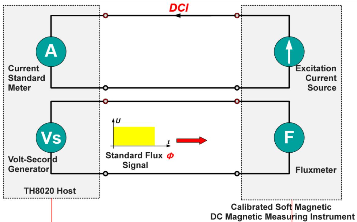
**Calibrated Soft Magnetic DC Magnetic Measuring Instrument**
