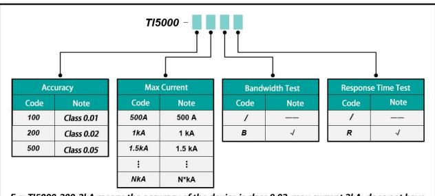
E.g: TI5000-200-2kA means the accuracy of the device is class 0.02, max current 2kA, does not have the function of sensor test and response time test.
