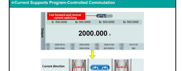
The device has a programmable switching output function in the positive and negative directions
