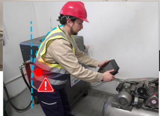
Traditional acoustic imager operation
